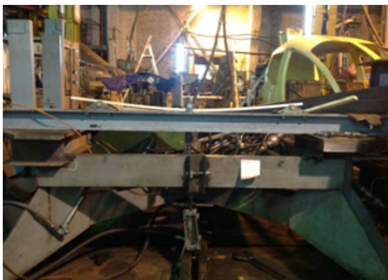
Figure 2. Testing stand imitating the ski work
